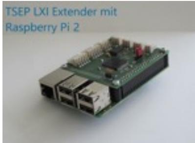
Due to this TSEP has developed the TSEP LXI Extender. Based on a low cost Linux system like Raspberry Pi or Cubieboard and the TSEP LXI Extender Interface Board now any  $\mu$ C can be connected via a standardised interface. Additionally it is of course possible to use the TSEP LXI Extender with customized hardware.
